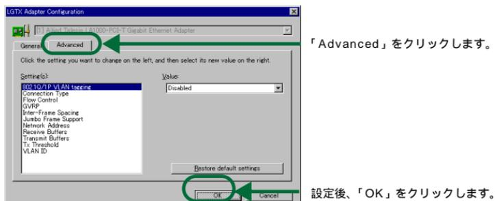
図 3.3.4 LGTX Adapter Configuration
