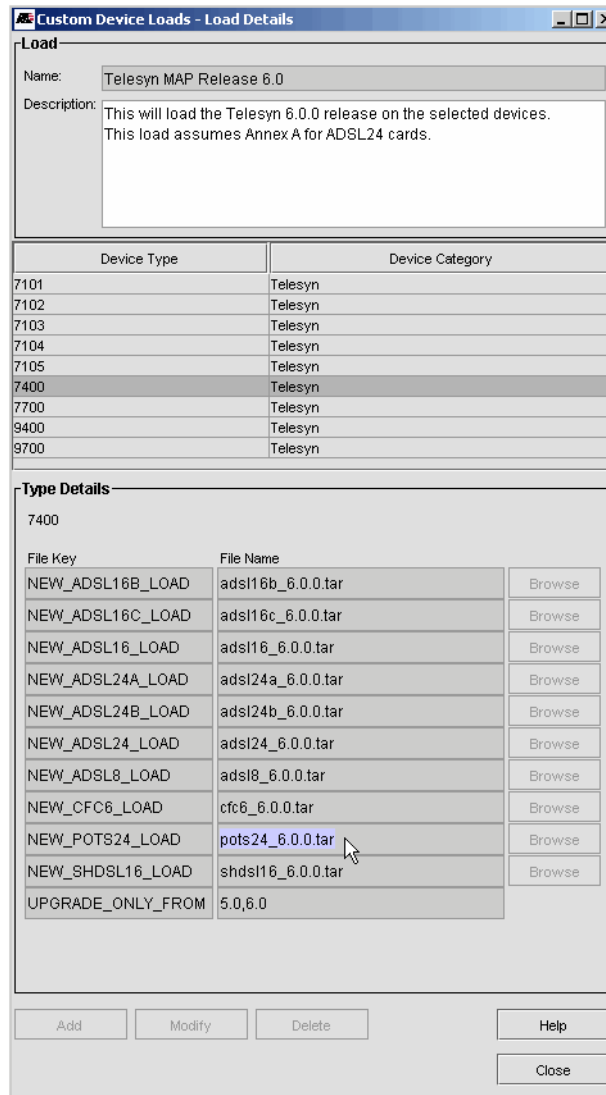
FIGURE 5-62 Details Display for Standard Load (Used to Create Custom Load of Only Certain Files)
